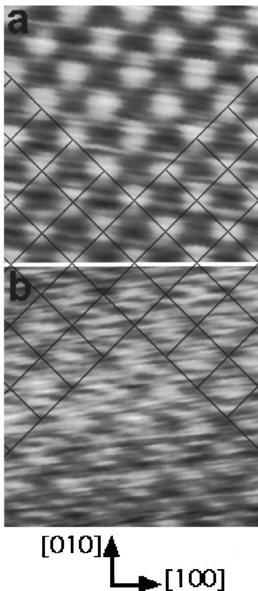
FIG. 6. Empty states (a), (+1.1 V sample bias, 1.0 nA tunneling current) and filled states (b), (-1.5 V sample bias, 1.0 nA tunneling current) atomically resolved STM images of the (100) surface of NiO. The two images have been presented so that the bright Ni sites seen in (a) are located between the bright O sites imaged in (b) (see text). The average corrugation heights are approximately 0.3 Å in (a) and 0.15 Å in (b).
