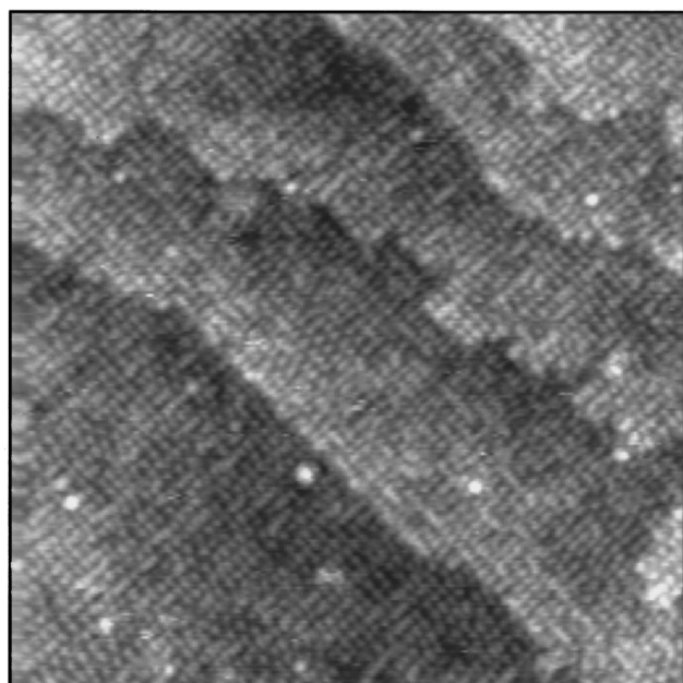
FIG. 3. Filled-state image of the Si(100) surface after exposure to 2 L of C 2 H 2 . This exposure resulted in saturation coverage and produced an ordered 2×2 overlayer. The image size is 300 × 300 Å 2 . The sample bias is -2.4 V.
