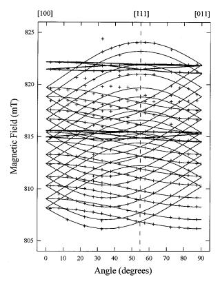
FIG. 2. Angular dependence of the Si-NL56 and Si-NL57 spectra measured for the  $^{109}$ Ag-doped sample. The bold and thin solid lines represent fits to the experimental data (+) according to Eq. (1) for spectrum Si-NL56 and Eq. (2) for Si-NL57, respectively. The microwave frequency is  $\nu$ =22.8697 GHz.
