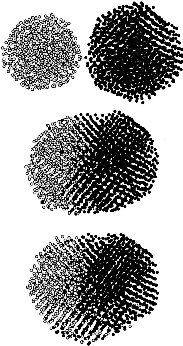
FIG. 11. Configuration of the 767+1505 liquid-solid system at three different times: 0, 1 ns, and 10 ns (top to bottom).
