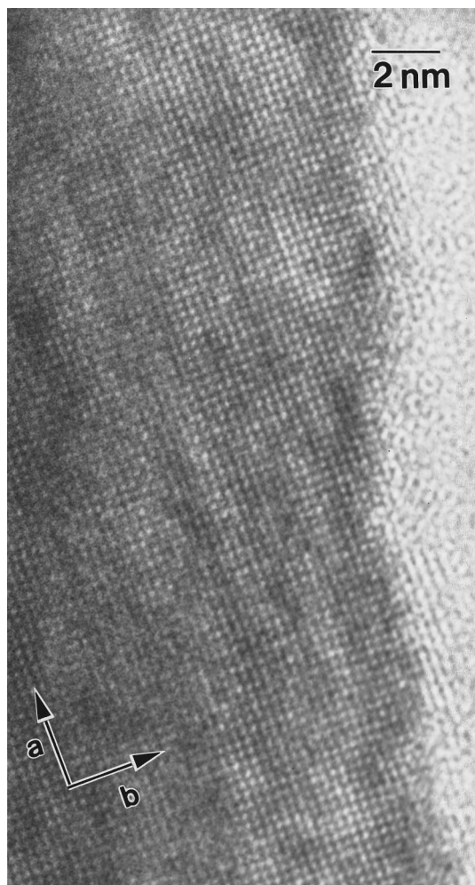
FIG. 2. A high-resolution TEM image of the a - b plane surface of a Pb-substituted Bi2212 crystal.
