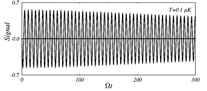
FIG. 2. The microwave induced electron-spin-resonance Rabi oscillation of a Bose gas above the critical temperature for BEC. The temperature for the gas is chosen to be  $T=0.1 \mu\text{K}$ .
