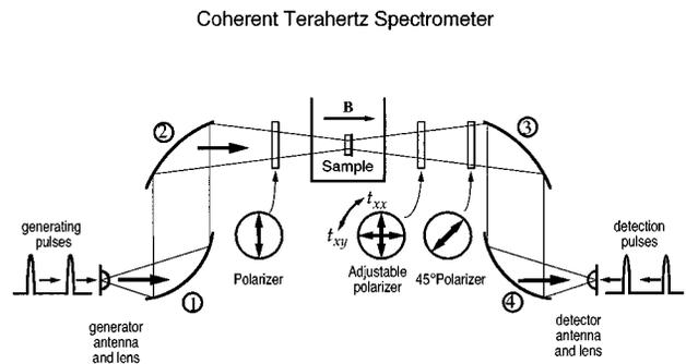
FIG. 1. Time-domain spectrometer for measurement of the complex transmission tensor in the presence of a magnetic field. Diagonal  $t_{xx}$  and off-diagonal  $t_{xy}$  components are selected by rotating the analyzing polarizer through  $90^\circ$ . The effect of linear birefringence is removed by reversing the field direction.
