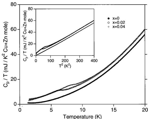
FIG. 4. Total specific heat divided by temperature  $C_p/T$  vs  $T$  and  $T^2$  (inset) of  $\text{Sr}(\text{Cu}_{1-x}\text{Zn}_x)_2\text{O}_3$  ( $x=0, 0.02$ , and  $0.04$ ).
