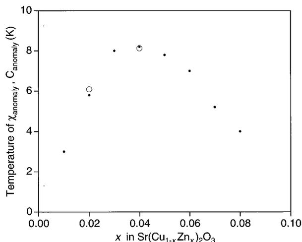
FIG. 3. Temperatures where susceptibility (closed circles) and specific heat (open circles) reach maxima are plotted against Zn content.
