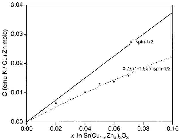
FIG. 2. Estimated Curie constant (●) of  $\text{Sr}(\text{Cu}_{1-x}\text{Zn}_x)_2\text{O}_3$  plotted against Zn content. The solid line stands for the Curie constant expected from an assumption that every Zn ion produces a spin 1/2. See the text about the dotted line.
