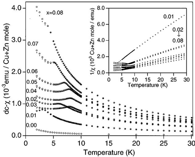
FIG. 1. Temperature dependence of the dc magnetic susceptibility of  $\text{Sr}(\text{Cu}_{1-x}\text{Zn}_x)_2\text{O}_3$  measured in an external field of 100 Oe on heating (closed circles) and cooling (open circles). Inset shows temperature dependence of the inverse susceptibility for  $x=0.01$  to 0.08 from the top to the bottom.
