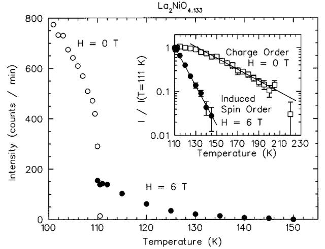
FIG. 4. Temperature dependence of the intensity of the magnetic peak at  $\mathbf{Q}=(1-\epsilon,0,1)$  measured with  $H=0$  (open circles) and  $H=6$  T (filled circles). Below  $\sim 109$  K the magnetic peaks become independent of field. Inset: logarithm of normalized intensity vs temperature for the magnetic peak at  $H=6$  T (filled circles), and for the charge-order peak at  $(4-2\epsilon,0,1)$  (open squares, from Ref. 20). Lines through points are linear fits, as discussed in the text.
