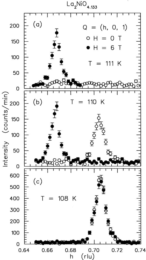
FIG. 3. Elastic scans along  $\mathbf{Q}=(h,0,1)$  in zero field (open circles) and in a magnetic field of 6 T (filled circles). Scans were measured at temperatures of 111 K (a), 110 K (b), and 108 K (c).
