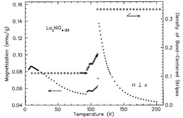
FIG. 2. Bulk magnetization measured (on warming, after zero-field cooling) with an applied field of 1 T aligned parallel to the  $\text{NiO}_2$  planes (circles), and density of bond-centered stripes (squares), which is equal to  $4\epsilon - 1$ , where values of  $\epsilon$  are taken from Ref. 20.
