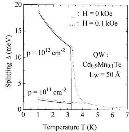
FIG. 2. Temperature dependence of the heavy-hole spin splitting in the 50 Å quantum well of  $\text{Cd}_{0.9}\text{Mn}_{0.1}\text{Te}$  for two values of the hole areal densities  $p$  and the magnetic fields  $H$ . Provided that the holes are delocalized, the mean-field value of ferromagnetic critical temperature  $T_c \approx 3$  K does not depend on  $p$ . By contrast, the saturation value of the spin splitting is seen to increase with  $p$ .
