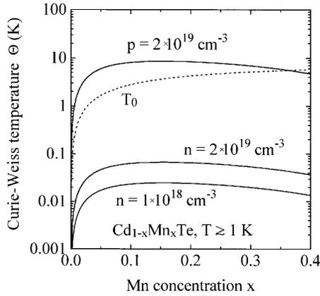
FIG. 1. Mean-field value of the Curie-Weiss temperature  $\Theta$  of Eq. (3) for  $p$ - and  $n$ -type  $\text{Cd}_{1-x}\text{Mn}_x\text{Te}$ , compared to antiferromagnetic temperature  $T_0(x)$ . Ferromagnetic phase transition may occur at  $T = \Theta - T_0$ . Material parameters as determined at 1.7 K were adopted for the calculation.
