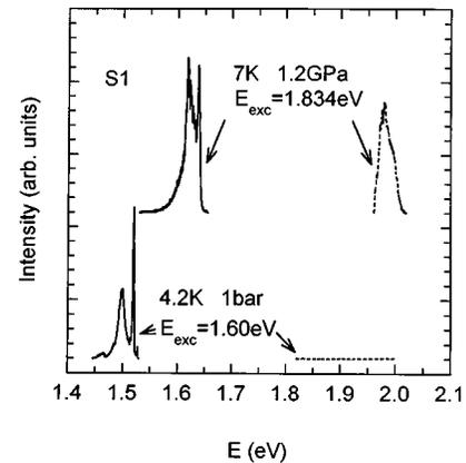
FIG. 4. A comparison between the emission spectra of S1 measured at 1 bar and at 1.2 GPa. The up-converted spectra are represented by broken curves. Notice that the GaAs emission peaks are shifted to higher energy by pressure.
