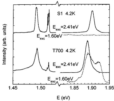
FIG. 1. Emission spectra of T700 and S1 in both the GaAs region (around 1.50-eV region) and the GaInP<sub>2</sub> region at 0 T and 1 bar. The broken curves show the up-converted photoluminescence.
