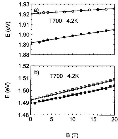
FIG. 3. Plot of the deconvoluted peak energies (see text) vs  $B$  in T700 for (a) the up-converted spectra of GaInP<sub>2</sub> and (b) the 1.49-eV structure in GaAs. The solid lines are least-square fits of the data points with a straight line.
