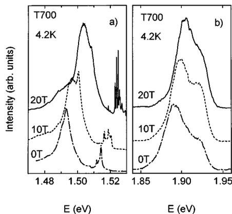
FIG. 2. The magnetic-field-dependent emission spectra of T700 in (a) the GaAs band-gap region and (b) the GaInP<sub>2</sub> band-gap region when excited by photons of 1.60 eV.
