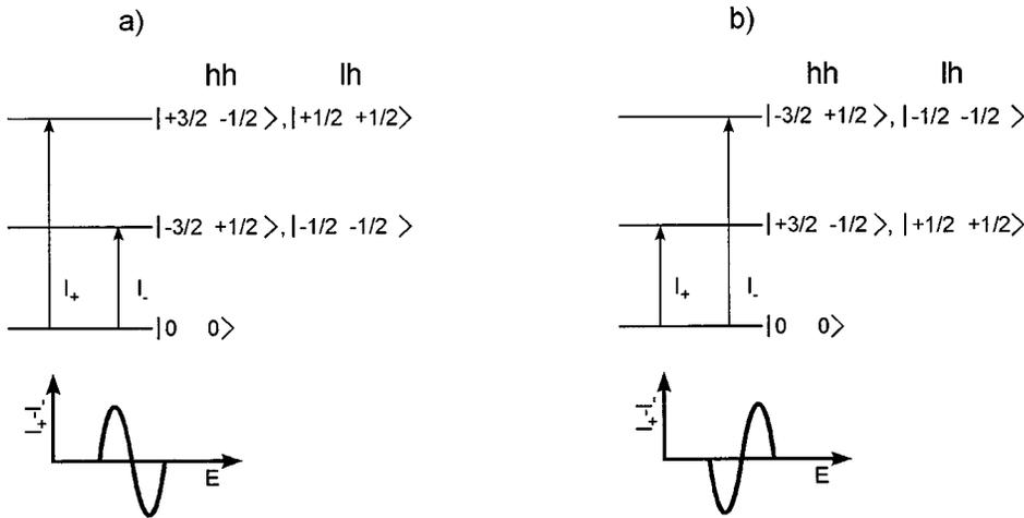
FIG. 5. The schematic structure of the possible transitions: (a) schemes leading to a positive left wing for the MCD signal. (b) schemes leading to a positive right wing for the MCD signal. The allowed optical transitions are marked with arrows.
