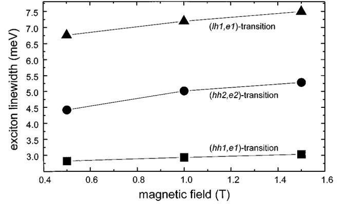
FIG. 3. Half-width of the ( $hh1,e1$ ), the ( $lh1,e1$ ) and the ( $hh2,e2$ ) transitions determined from the energy separation of the maximum and minimum of the MCD spectra.
