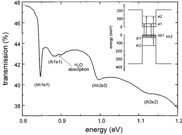
FIG. 1. Transmission spectra of the  $\text{In}_x\text{Ga}_{1-x}\text{As}$  quantum wells. The observed transitions are as follows: first heavy hole to first electron ( $hh1,e1$ ), first light hole to first electron ( $lh1,e1$ ), second heavy hole to second electron ( $hh2,e2$ ), and second light hole to second electron ( $lh2,e2$ ). The inset shows the self-consistently calculated band structure.
