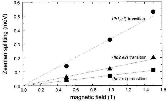
FIG. 4. Zeeman splitting of the different transitions as a function of the magnetic field.
