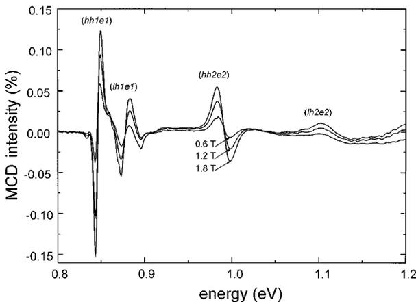
FIG. 2. MCD spectra of the  $\text{In}_x\text{Ga}_{1-x}\text{As}$  quantum wells at different magnetic fields. All the transitions in Fig. 1 are observed to have a derivative line shape.
