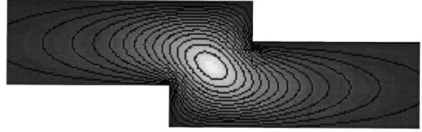
FIG. 10. Contour plot of the calculated wave function for the electron bound state in wire with the aspect ratio  $R=1.5$ , showing a single maximum in the center of the bend region.
