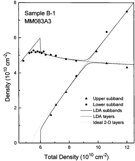
FIG. 2. Experimental results and the LDA simulation for a dilute bilayer electron system. The experimental data were taken at 25 mK. Note the excellent agreement at all points except those where the discontinuous charge transfer is predicted.
