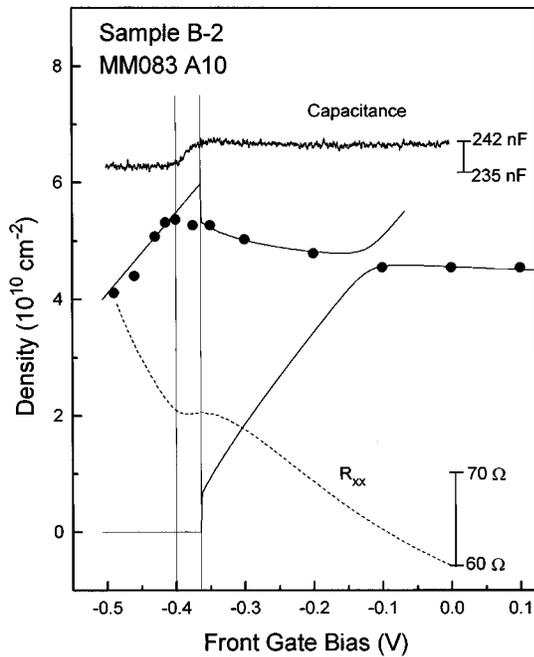
FIG. 3. Experimental data taken at 0.3 K, showing subband density  $R_{xx}$  and capacitance as a function of  $V_{FG}$ . The capacitance and  $R_{xx}$  were measured at  $B=0$ . The LDA simulation was fitted to the experimental data. All three data sets show that the front layer depletion happens at a more negative  $V_{FG}$  than the LDA predicts.
