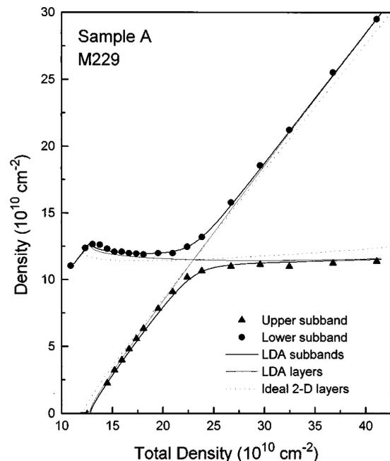
FIG. 1. The measured (symbols) and LDA simulation results (thick solid curves) for the subband densities in a double-quantum-well sample. Note the excellent agreement between the experimental data and the LDA results over the whole density range. The solid curves show the layer densities deduced from the LDA simulation. The dotted curves are from a simulation where the layers are taken to be ideal two-dimensional sheets.
