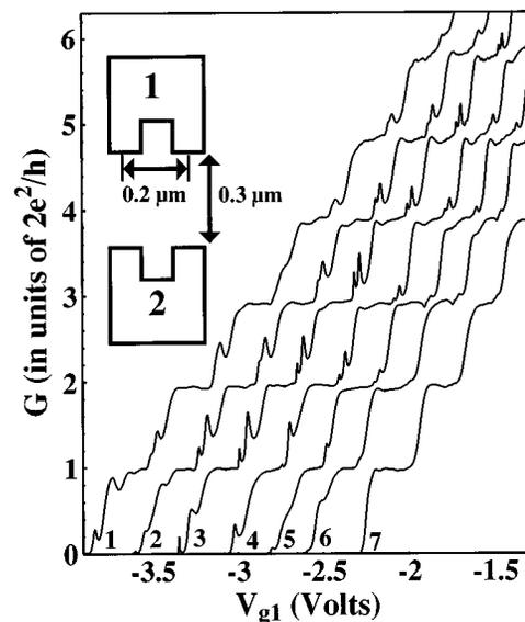
FIG. 1.  $G(V_{g1})$  when the conduction path is electrostatically shifted by applying various gate voltages to gate 2. Traces 1 to 7:  $V_{g2} = -1.3, -1.5, -1.7, -1.9, -2.1, -2.3,$  and  $-2.6 \text{ V}$ , respectively. The inset shows the Schottky gate geometry.
