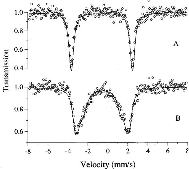
FIG. 4. Mössbauer transmission spectra of thin foils of iron metal and Invar alloy measured with radiation from the SMS. (A) iron foil of  $1.3 \mu\text{m}$  thickness, magnetized:  $H_{\text{ext}} \parallel h_1$ ; (B) Invar foil of  $1 \mu\text{m}$  thickness, magnetized:  $H_{\text{ext}} \parallel h_1$ . The solid lines are fits using the transmission integral. The field strength distribution is simulated by three Lorentzians.
