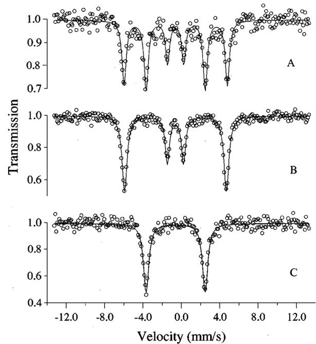
FIG. 3. Mössbauer transmission spectra of an  $^{57}\text{Fe}$  foil of 1.3  $\mu\text{m}$  thickness measured with radiation from the SMS. (A) foil nonmagnetized; (B) foil magnetized:  $H_{\text{ext}} \perp h_1$  and  $H_{\text{ext}} \perp k_1$ ; and (C) foil magnetized:  $H_{\text{ext}} \parallel h_1$ . The solid lines are fits using the transmission integral with 100% linearly polarized and fully recoilless radiation.
