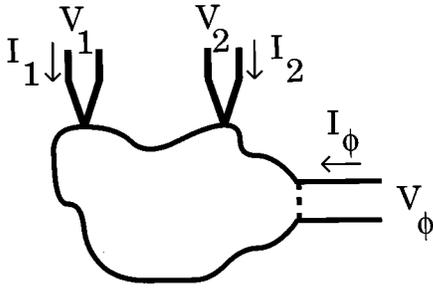
FIG. 1. Chaotic cavity, connected to current source and drain reservoirs (1 and 2), and to a voltage probe ( $\phi$ ). The voltage probe contains a tunnel barrier (dotted line). The voltage  $V_\phi$  is adjusted such that  $I_\phi=0$ .
