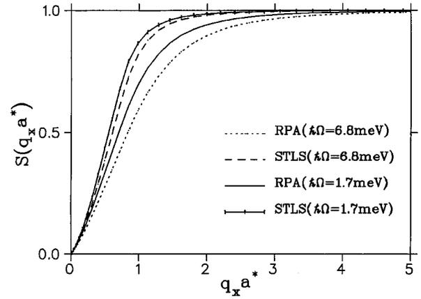
FIG. 4. Structure factor for a quasi-1D electron gas in a semiconductor GaAs quantum wire for the lowest subband calculated in a two-subband model where one subband is filled as a function of the wave vector  $q_x a^*$ . Sizable differences can be seen in comparison to the RPA results mainly for a subband separation energy of  $\hbar\Omega = 6.8$  meV.
