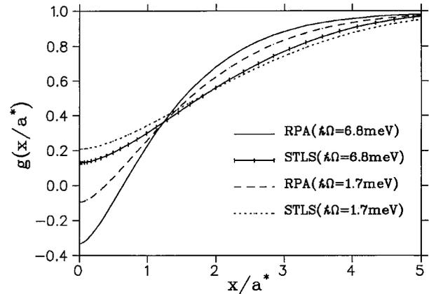
FIG. 5. Pair-correlation function for a quasi-1D electron system in a GaAs quantum wire in which only the lowest subband is occupied by electrons as a function of the wave vector  $q_x a^*$ . The RPA results are shown for comparison with the self-consistent-field approximation. For the subband separation energies  $\hbar\Omega$  the STLS-gives a positive value, while RPA gives a negative nonphysical result for the pair-correlation function at  $x=0$ .
