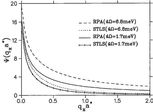
FIG. 3. Effective electron-electron potential for the first subband as calculated within the self-consistent-field approximation for different subband separation energies  $\hbar\Omega$  of GaAs quantum wires as a function of the wave vector  $q_x a^*$ . The RPA results are also shown for comparison.
