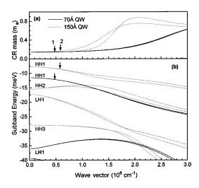
FIG. 5. (a) Semiclassical CR mass, as a function of wave vector, obtained from the zero-field subband dispersion and Eq. (2) (see text) for samples 1 (solid) and 3 (dotted). Arrows indicate the Fermi wave vector for sample 1 (arrow 1) and sample 3 (arrow 2). (b) Zero-field subband dispersions for samples 1 (solid) and 3 (dotted). The subbands are labeled according to their wave-function character at zero wave vector. Energy is measured relative to the valence-band edge.
