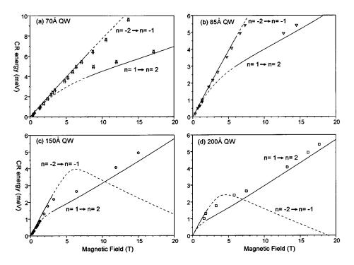
FIG. 7. The measured CR energies are plotted for each field value. The transition energy for the two transitions  $n=-2 \rightarrow n=-1$  and  $n=1 \rightarrow n=2$ , as calculated in the model described in the text, are plotted for comparison. Where the transition is forbidden (at zero temperature) through either an empty initial state or a completely filled final state, the transition energy is plotted as a dashed line. (a)–(d) show results for samples 1–4, respectively.
