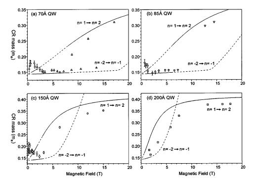
FIG. 8. The same data as plotted in Fig. 7 are shown in the form of CR mass  $(=eB/\omega_c)$  as a function of magnetic field. (a)–(d) show results for samples 1–4, respectively.
