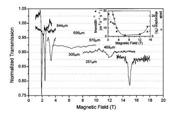
FIG. 3. CR spectra for sample 3 are plotted at a range of FIR laser wavelengths. In the inset are plotted the inverse linewidths (solid triangles) and peak resonant absorptions (open triangles) for sample 3.
