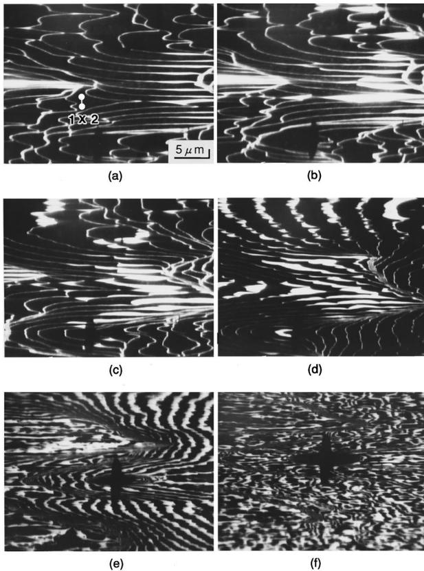
FIG. 3. REM images of a Si(001)  $1 \times 2$  surface heated to (a) 980 °C, (b) 1000 °C, (c) 1025 °C, (d) 1070 °C, (e) 1100 °C, and (f) 1140 °C. The images were observed after the sample was cooled to room temperature.
