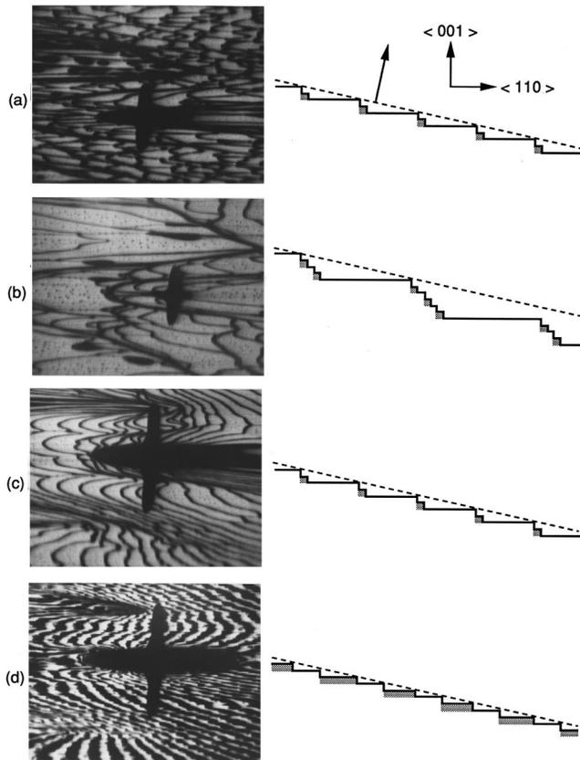
FIG. 8. Distribution of steps on a  $2\times 1$  terrace: (a) dispersion of pairs of steps at temperatures below  $850^\circ\text{C}$ , (b) aggregation of steps at temperatures near  $950^\circ\text{C}$ , (c) dispersion of pairs of steps at temperatures between  $1000^\circ\text{C}$  and  $1070^\circ\text{C}$ , and (d) dispersion of steps at temperatures between  $1070^\circ\text{C}$  and  $1100^\circ\text{C}$ .
