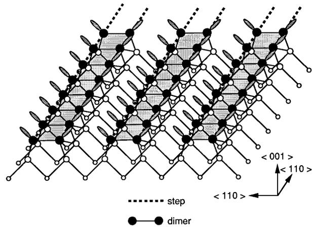
FIG. 6. Each dimer row corresponds to an atomic step. At high temperatures, Si atoms evaporate from every dimer row.
