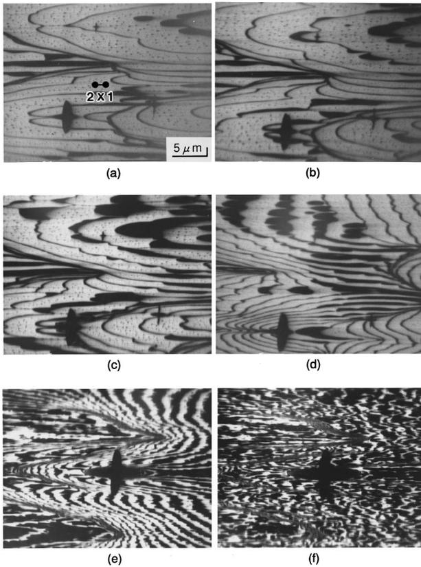
FIG. 1. REM images of a Si(001)  $2\times 1$  surface heated to (a) 980 °C, (b) 1000 °C, (c) 1025 °C, (d) 1070 °C, (e) 1100 °C, and (f) 1140 °C. The images were observed after the sample was cooled to room temperature.
