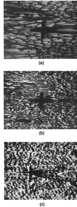
FIG. 2. REM images of a surface (a) before heating, (b) after 60 s of heating at 1140 °C, and (c) after flash heating. The images were observed after the sample was cooled to room temperature.
