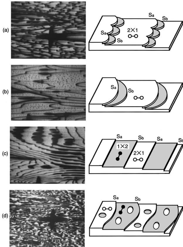
FIG. 5. Surface topographies of a Si(001)  $2\times 1$  sample heated to (a) below  $850^\circ\text{C}$ , (b) between  $900^\circ\text{C}$  and  $1000^\circ\text{C}$ , (c) between  $1000^\circ\text{C}$  and  $1100^\circ\text{C}$ , and (d) above  $1100^\circ\text{C}$ .
