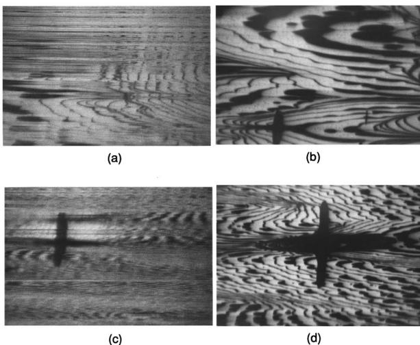
FIG. 4. *In situ* observations of a Si(001) surface: (a) the REM image obtained at 1050 °C and (b) the image after cooling the sample to room temperature; (c) the image obtained at 1090 °C and (d) the image after cooling it to room temperature.
