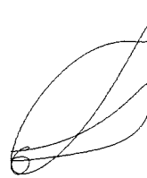
FIG. 3. Series of phase plots obtained by increasing the microwave frequency from 4.0 to 4.9 GHz. The Gunn mode maintains a 1:2 frequency-locked solution up to microwave frequencies of approximately 4.8 GHz. At f_{dc} = 4.9 GHz, a quasiperiodic solution (or a periodic solution with a period longer than 2 ns) is observed.
