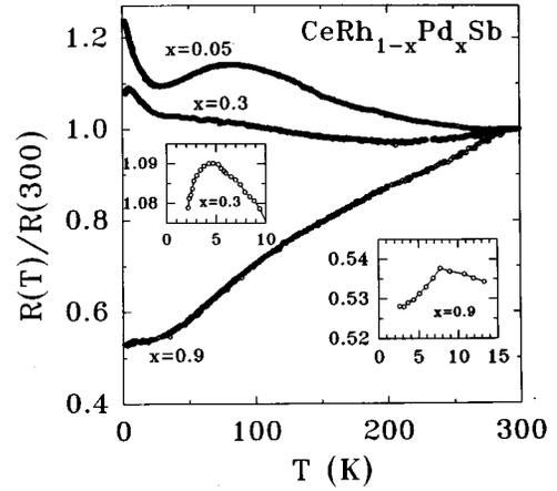
FIG. 3. Electrical resistivity  $\rho$  vs temperature  $T$  for  $\text{CeRh}_{1-x}\text{Pd}_x\text{Sb}$  ( $x=0.05, 0.3,$  and  $0.9$ ). Insets show the low-temperature drop in  $\rho$  for  $x=0.3$  and  $0.9$ .
