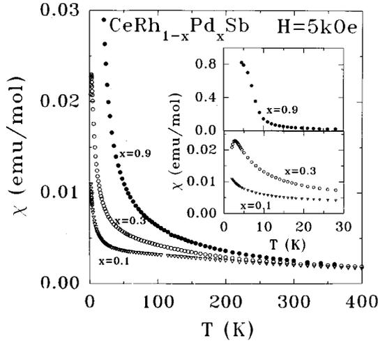
FIG. 1. Magnetic susceptibility  $\chi$  vs temperature  $T$  for  $\text{CeRh}_{1-x}\text{Pd}_x\text{Sb}$  ( $x=0.1, 0.3,$  and  $0.9$ ) compounds. Inset shows the low-temperature behavior.
