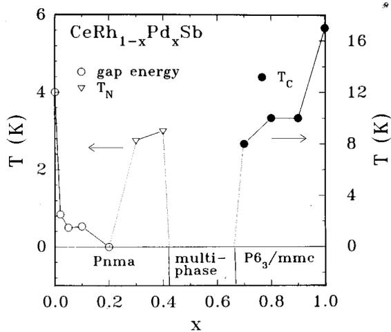
FIG. 4. Phase diagram of  $\text{CeRh}_{1-x}\text{Pd}_x\text{Sb}$  for  $0 \leq x \leq 1$ . In the figure,  $\Delta$  refers to the gap energy,  $T_N$  to the Néel temperature, and  $T_C$  to the Curie temperature. The lines are drawn as a guide to the eye.
