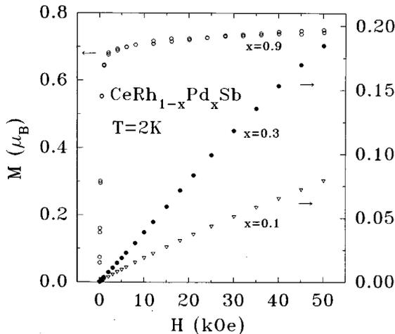
FIG. 2. Magnetization  $M$  vs field  $H$  for  $\text{CeRh}_{1-x}\text{Pd}_x\text{Sb}$  ( $x=0.1, 0.3,$  and  $0.9$ ). The left-hand side scale is for  $x=0.9$  sample, and the right-hand side scale is for  $x=0.1$  and  $0.3$  samples.
