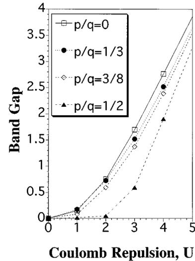
FIG. 3. Band gap vs Coulomb repulsion energy  $U$  as a function of magnetic flux per plaquette,  $\phi$ .
