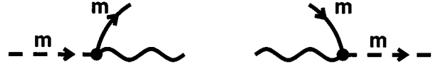
FIG. 1. Vertices for the Anderson model. A dashed line represents the naked propagator of the occupied f^1 configuration with internal quantum number m . A wavy line represents the naked propagator of the unoccupied f^0 configuration. A solid line represents the propagator of a conduction electron with internal quantum number m . Every diagram has a spine of alternating wavy and dashed impurity propagators. The conduction-electron propagators carry no self-energy (Ref. 14).
