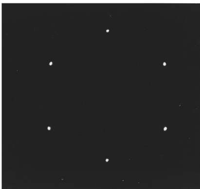
FIG. 4. Photograph of the LEED pattern of 3-ML Fe/2-ML Ni/W(110), for a primary beam energy of 96 eV. The orientation of the tungsten substrate and Ni film in direct space is as the NW unit cells in Fig. 1.
