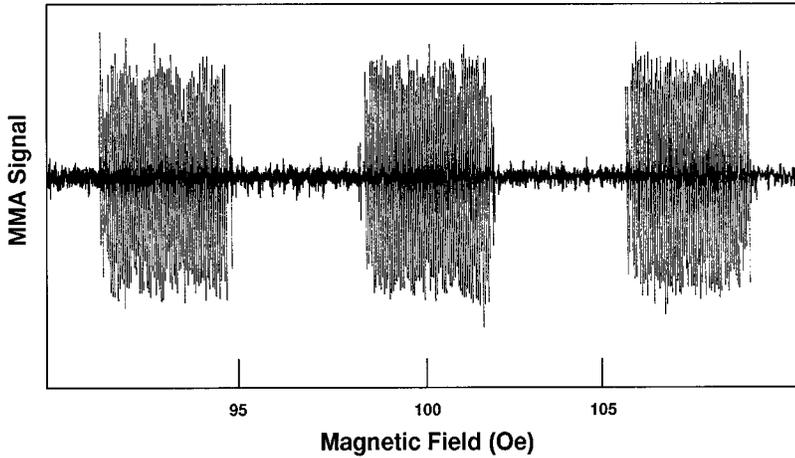
FIG. 6. A portion of a Josephson junction spectrum with a line separation of about 50 mOe is shown over a range of about 20 Oe at 4.0 K and 9.3 GHz with a 100 kHz modulation field of 5 mOe and a microwave power of 0.45 mW.
