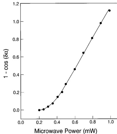
FIG. 3. A plot of  $(1 - \cos\delta\alpha)$  vs  $P$ , where  $\delta\alpha = \pi\delta H/\Delta H$ .  $H$  is shown for the data of Table I.
