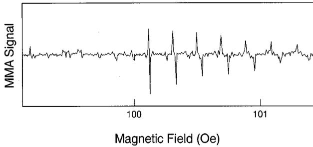
FIG. 4. A Josephson junction spectrum in which  $\delta H$  increases in field from line to line is shown for 9.3 GHz and 3.8 K with a 100 kHz peak-to-peak modulation field of 5 mOe and a microwave power of 0.45 mW.
