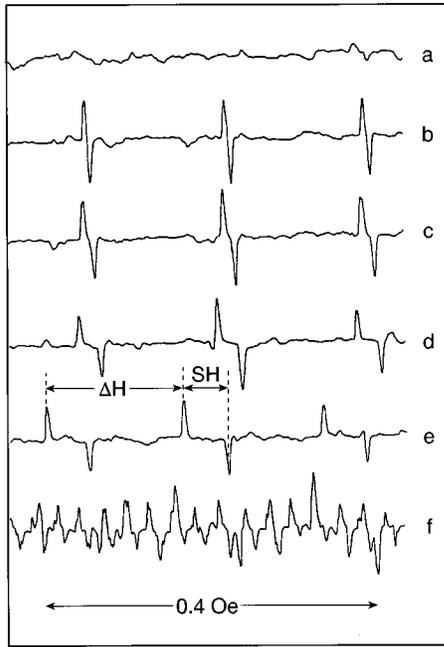
FIG. 1. Josephson junction spectra near 100 Oe from a scratched Nb wire are shown at 9.3 GHz and 3.9 K for microwave power values of 0.20 mW (curve *a*), 0.25 mW (curve *b*), 0.30 mW (curve *c*), 0.40 mW (curve *d*), 0.60 mW (curve *e*), and 0.80 mW (curve *f*). The separations  $\delta H$  and  $\Delta H$  are illustrated in curve *e*. The 100 kHz modulation field in each case has a peak-to-peak value of 5 mOe.
