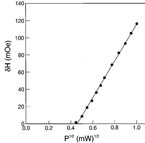
FIG. 2. A plot of  $\delta H$  vs  $P^{1/2}$  is shown for the data of Table I. The straight line represents a least-squares fit of the data to Eq. (4) with  $a = 215$  mOe/(mW)<sup>1/2</sup> and  $b = -98$  mOe.
