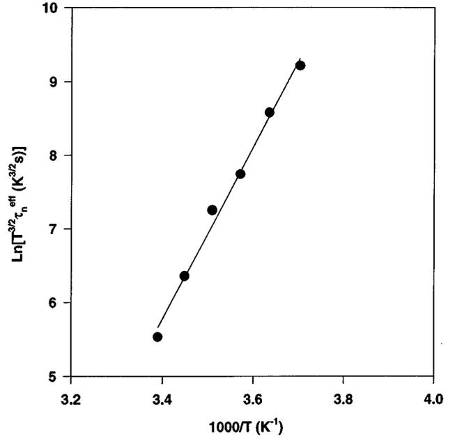
FIG. 4. Modified Arrhenius plot for the transient SPV data fitted from Fig. 2. The energy depth of the dominant traps is found to be  $E_t=0.99\pm 0.05$  eV.
