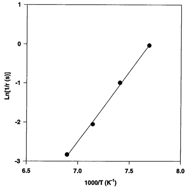
FIG. 6. Arrhenius plot for the data fitted from Fig. 5. The EL2\* thermal recovery rate is given by  $1.9\times 10^{12} \exp(-0.32 \text{ eV}/kT) \text{ s}^{-1}$ .
