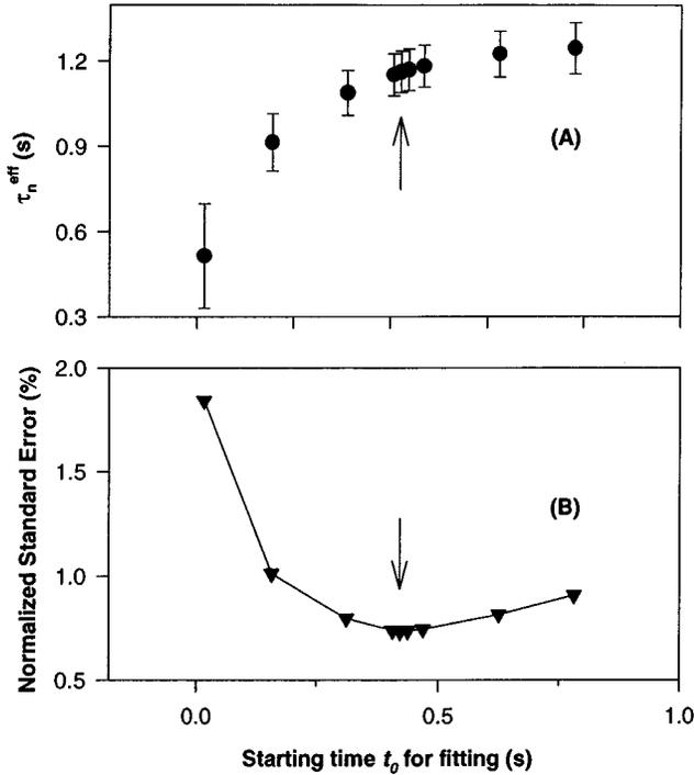
FIG. 3. Curve-fitting results for the effective time constant  $\tau_n^{\text{eff}}$  of reciprocal SPV transients at  $T=275$  K using different starting time  $t_0$  (see text) with enlarged error bar (by factor of 50) (A), and the normalized standard error [i.e., coefficient of variable (CV%)] vs  $t_0$  (B). The minimum CV% of 0.732% is found at  $t_0=422$  ms (marked with arrows), and the corresponding  $\tau_n^{\text{eff}}$  is 1.163 g.
