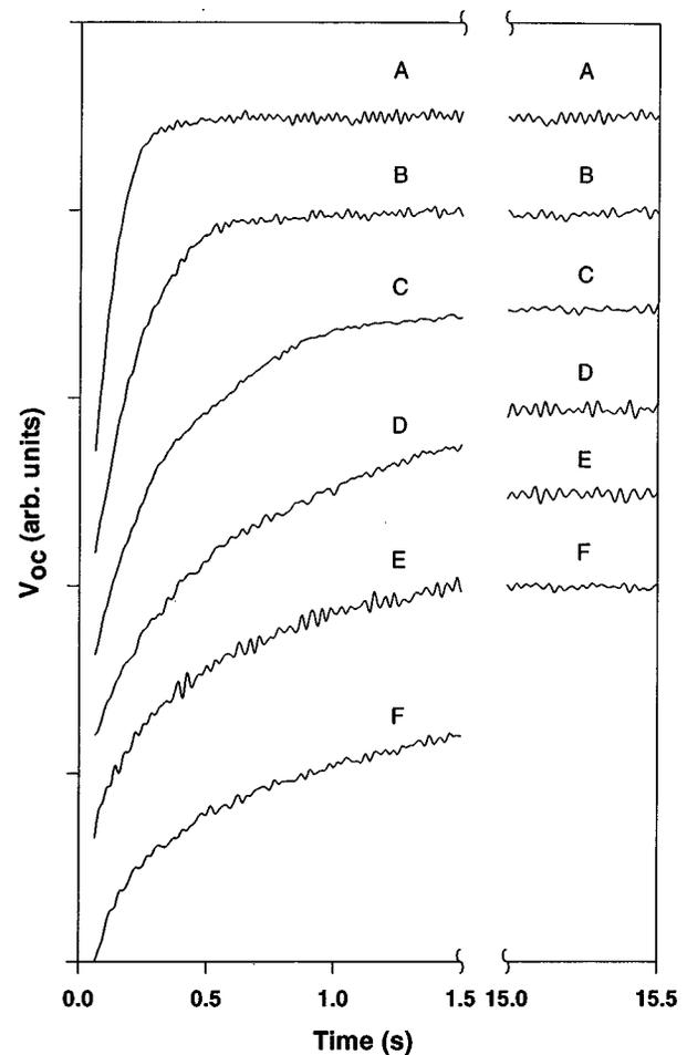
FIG. 2. Surface photovoltage  $V_{oc}$  transients for undoped semi-insulating GaAs as a function of time and optical bias at temperatures: 259 K (A), 290 K (B), 285 K (C), 280 K (D), 275 K (E), and 270 K (F).
