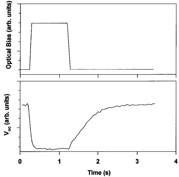
FIG. 1. Typical photovoltage transient waveform (A) for undoped semi-insulating GaAs at  $T=280$  K, due to the optical bias pulse (B).
