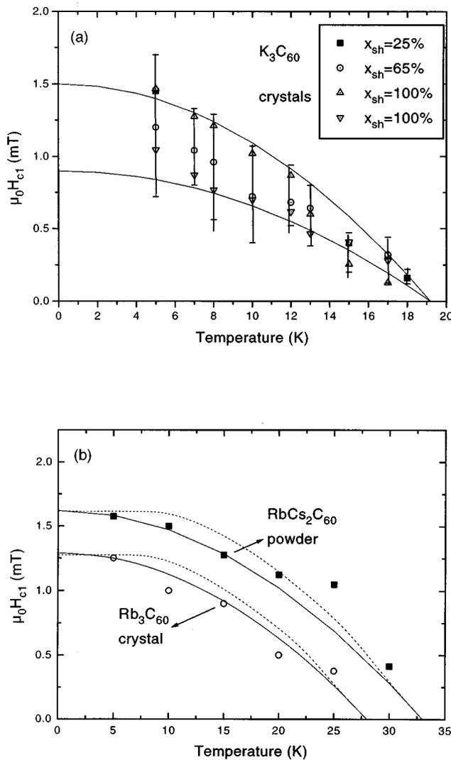
FIG. 3. Temperature dependence of the lower critical field of (a)  $K_3C_{60}$  crystals; (b)  $Rb_3C_{60}$  crystal (open circles) and  $RbCs_2C_{60}$  powder (solid squares). Solid lines correspond to Eq. (2) and dashed lines correspond to the weak-coupling BCS theory.
