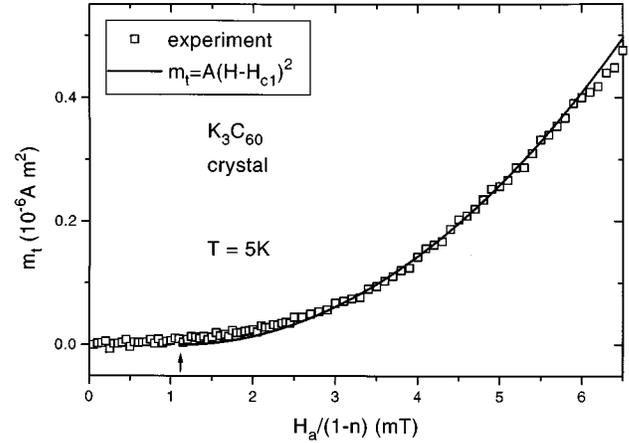
FIG. 2. Field dependence of the trapped magnetic moment of the  $K_3C_{60}$  single crystal at  $T=5$  K. The solid line corresponds to the equation  $m_t = A(H - H_{c1})^2$ .
