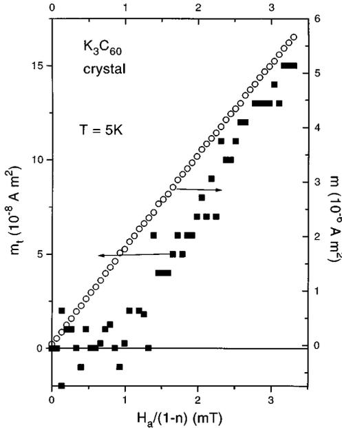
FIG. 1. Field dependence of the trapped magnetic moment (solid squares) and of the magnetic moment (open circles) of the  $K_3C_{60}$  single crystal taken at  $T=5$  K.
