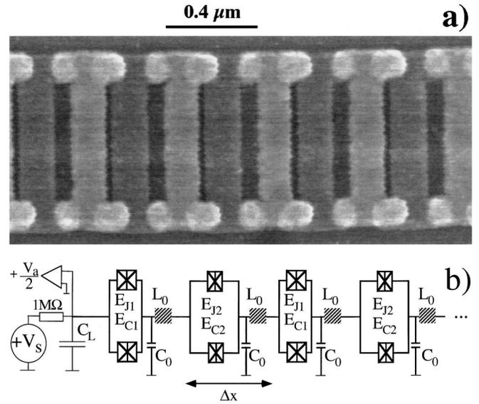
FIG. 1. (a) A SEM micrograph of a section of the array of SQUID's showing the alternating loop areas; and (b) the equivalent circuit showing one side of the symmetric bias arrangement.
