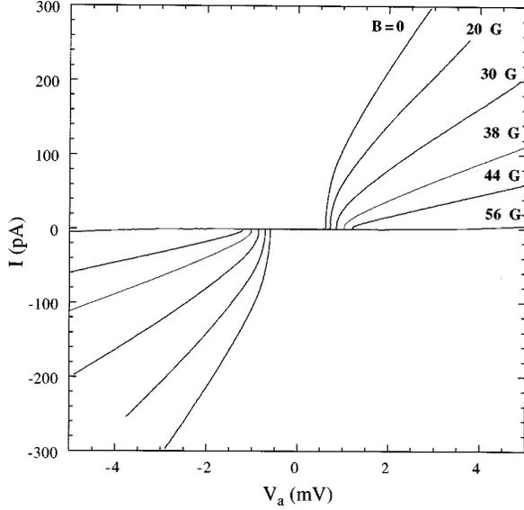
FIG. 2. The  $I$ - $V$  characteristic of the array for several magnetic fields. A distinct threshold voltage is seen, which depends on magnetic field.
