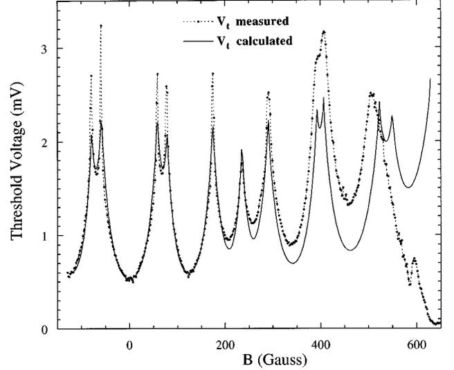
FIG. 3. The threshold voltage is shown versus magnetic field. The calculated curve explains the measured threshold voltage as being the injection voltage for a Cooper-pair charge soliton.
