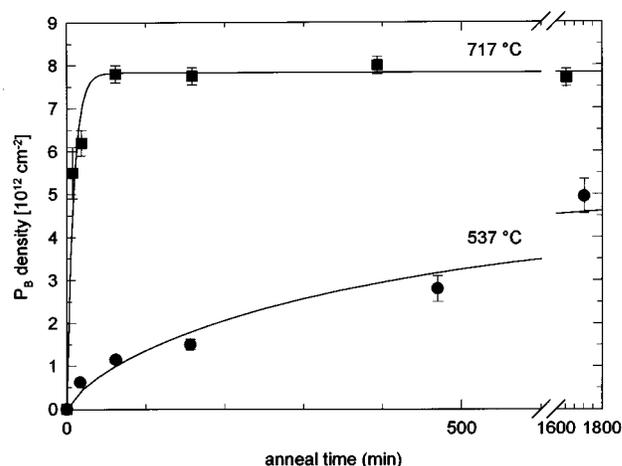
FIG. 2. Isothermal production of (ESR-active)  $P_b$  defects in standard (111) Si/SiO<sub>2</sub> (1.1 atm O<sub>2</sub>;  $\sim 967^\circ\text{C}$ ;  $d_{\text{ox}} \approx 42$  nm). For each  $T$ , data are obtained through cumulative stepwise annealing in vacuum of one sample initially exhaustively passivated in H<sub>2</sub> (1.1 atm H<sub>2</sub>; 405 °C;  $\sim 40$  min). The curves are guides to the eye.
