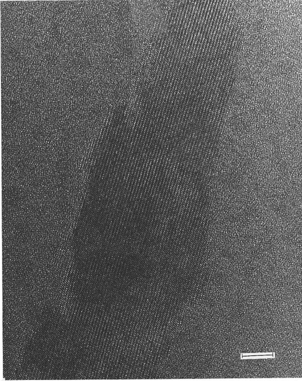
FIG. 5. High-resolution image of  $\text{Al}_{90}\text{La}_{10}$ , sample II. A grain of  $\text{Al}_{11}\text{La}_3$ , with a diameter of about 200 Å, is seen in the amorphous matrix. The unit length shown is 50 Å.
