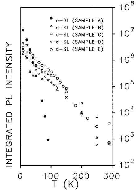
FIG. 2. Total PL intensity vs temperature for *o*-SL's (filled circles) and *d*-SL's (hollow symbols).
