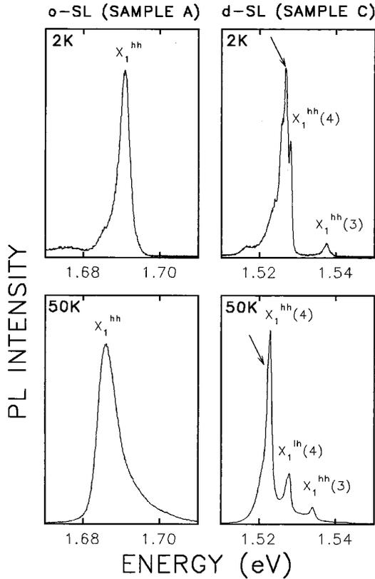
FIG. 1. PL spectra of an *o*-SL and a *d*-SL, at temperatures of 2 and 50 K. The redshift of the PL lines with  $T$  is evident.  $X_1^{\text{hh}}(i)$  and  $X_1^{\text{lh}}(i)$  indicate, respectively, heavy-hole and light-hole ground-state excitonic recombinations in the well of width  $L_{wi}$ . The arrows indicate the disorder-induced fine structure.
