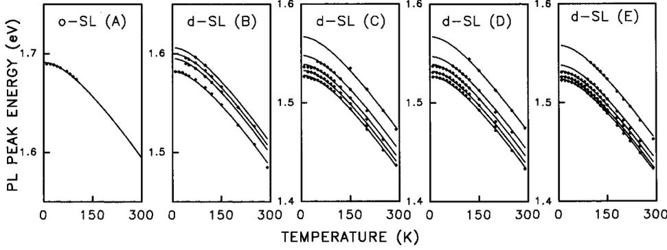
FIG. 3. The energies of the PL peaks of ordered and disordered SL's as a function of  $T$ . The observed redshift of the lines with increasing  $T$  has been fitted to the semiempirical Varshni relation (continuous lines) for the energy gap  $E_g(T)$  in GaAs.
