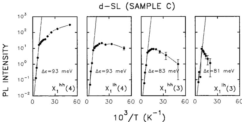
FIG. 4. Dependencies on  $T$  of the PL intensities of the various excitonic lines of a  $d$ -SL. The intensities of the PL lines were obtained by fitting the PL spectra. In the low- $T$  limit, propagation through variable range hopping is observed. In the high- $T$  limit an activationlike behavior is evident, and the activation energies  $\Delta\epsilon$ , obtained by fitting the data (continuous lines), are reported.  $X_1^{hh(i)}$  and  $X_1^{lh(i)}$  have the same meanings as in Fig. 1.
