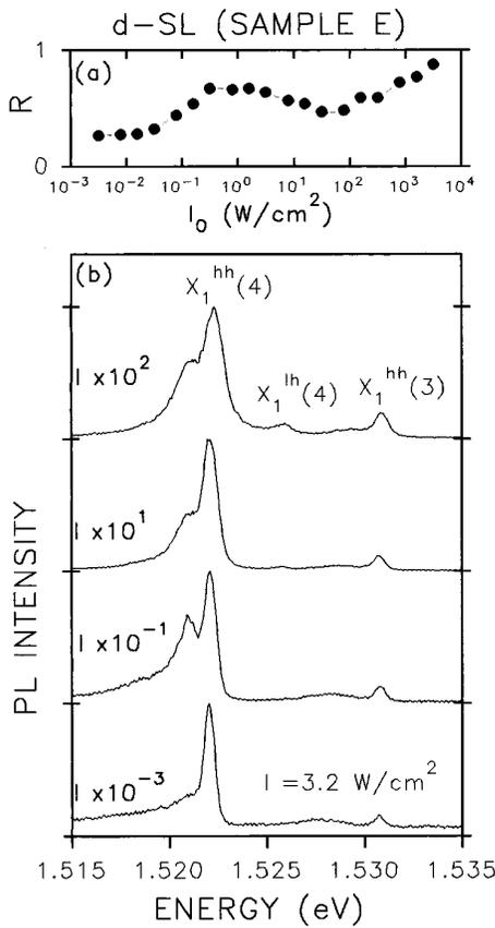
FIG. 5. (a) The intensity ratio  $R$  between the low- and high-energy parts of the PL emitted by the  $X_1^{hh}(4)$  subminiband, as a function of excitation intensity  $I_0$ . The observed nonmonotonic behavior is probably connected to the strong localization of the low-energy  $X$  states (see text). (b) PL spectra of a  $d$ -SL at different excitation intensities  $I_0$  measured on the same spot.  $X_1^{hh}(i)$  and  $X_1^{lh}(i)$  have the same meanings as in Fig. 1.
