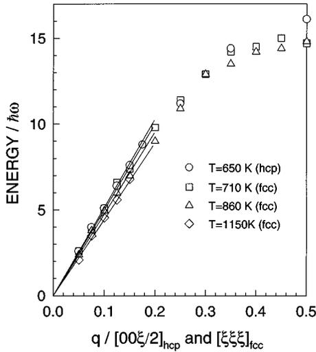
FIG. 2. Dispersion branch  $T_{100}[00\xi]_{\text{hcp}}$  at 650 K (circle), and  $T_{112}[\xi\xi\xi]_{\text{fcc}}$ , at 710 K (square), 860 K (triangle), and 115 K (cross) (all measured with sample 1).
