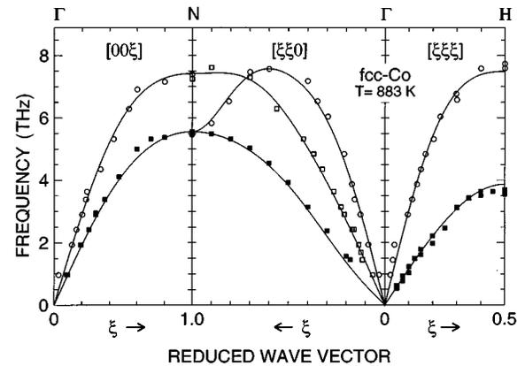
FIG. 1. Dispersion curve of fcc Co measured at 883 K on samples 1 and 2. The solid lines represent a Born–von Kármán fit including interactions up to the fourth-nearest neighbor.
