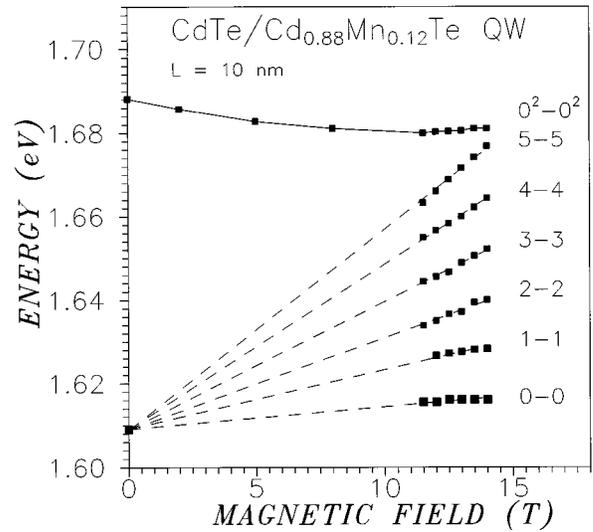
FIG. 6. Landau fan plot for allowed magnetoplasma transitions from a 10-nm CdTe QW.
