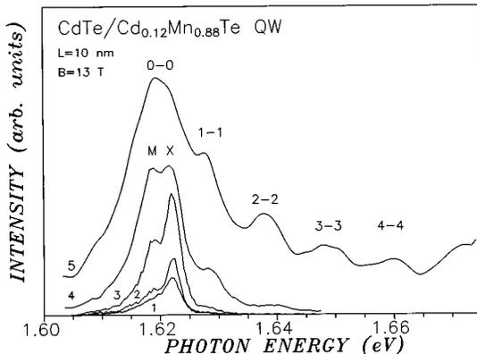
FIG. 5. Emission spectra from CdTe QW at  $T = 4.2$  K,  $B = 13$  T and various excitation densities.  $n_{e-h}(10^{12} \text{ cm}^{-2}) = 0.15$  (1),  $0.25$  (2),  $0.35$  (3),  $0.63$  (4), and  $1.8$  (5).
