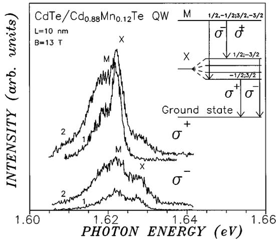
FIG. 4. Polarized spectra from a 10-nm thick CdTe QW at  $T = 4.2$  K,  $B = 13$  T and various excitation densities  $P=1$  (1) and  $0.3\mu\text{J}/\text{cm}^2$  (2). The inset displays the allowed transitions for excitons and excitonic molecules.
