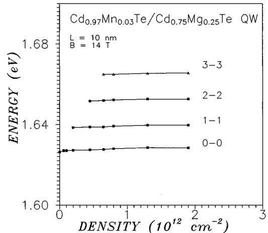
FIG. 3. Density dependence of LL transition energies in the first subband of a  $\text{Cd}_{0.97}\text{Mn}_{0.03}\text{Te}/\text{Cd}_{0.75}\text{Mg}_{0.25}\text{Te}$  QW at 14 T and  $T = 4.2$  K.
