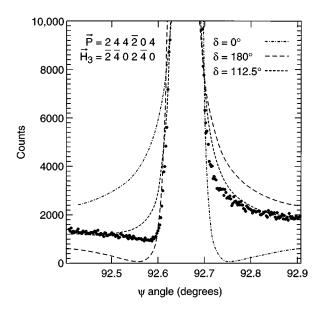
FIG. 3. The same as Fig. 2, except that the multiple diffraction peak (heavy dots) was truncated at the counting number of 10 000. The short-dashed line is a fit with a triplet invariant  $\delta$ =0°, and the long-dashed line is the one with  $\delta$ =180°. The small dashed line is the best fit, with  $\delta$ =112.5°.
