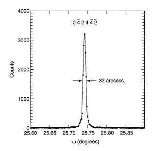
FIG. 1. Rocking curve of the  $(0\ \overline{4}\ 2\ 4\ \overline{4}\ \overline{2})$ . The counting time on each point was about 2 s. The increment  $\Delta\theta$  was  $0.002^{\circ}$ . The width of the rocking curve corresponds to the instrumental resolution.
