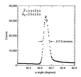
FIG. 2. Azimuthal plot of the  $(2 4 4 \overline{2} 0 4)$  reflection, a threebeam case. The simultaneous reflection **H** is the  $(\overline{2} \overline{4} 0 2 \overline{4} 0)$ . The x-ray energy is 7000 eV. The azimuthal angle is zero when the  $(0 0 0 0 \overline{1} 0)$  axis is in the scattering plane, mostly antiparallel to the incident beam, and the diffractometer angle  $\psi_0=249.771^\circ$ . The counting time on each point was about 1 s. The increment on  $\psi$  was  $0.002^\circ$ .
