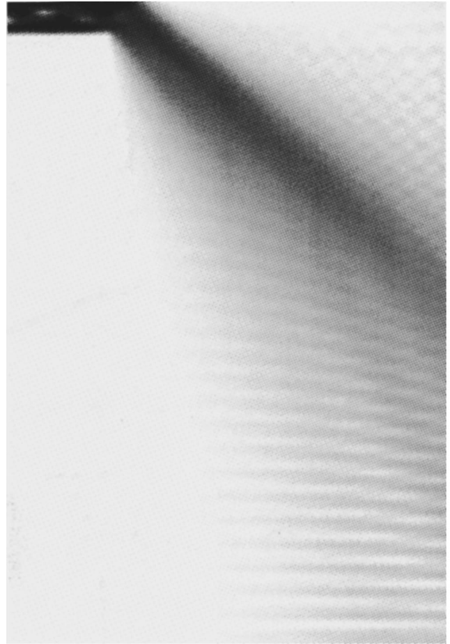
FIG. 7. Collimation of the beam is apparent in this picture, which describes the entry of particles from a point contact ( 0.05 \mu\text{m} wide) in which only two modes are allowed to propagate into a much wider quantum wire ( 0.8 \mu\text{m} wide).
