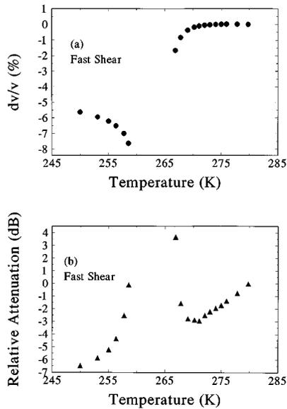
FIG. 4. Temperature dependence of the relative velocity,  $V_{44}$  (a) and the relative attenuation (b) associated with the elastic constant  $C_{44}$ . The gap in the data is due to the high attenuation associated with the transition to the intermediate phase.
