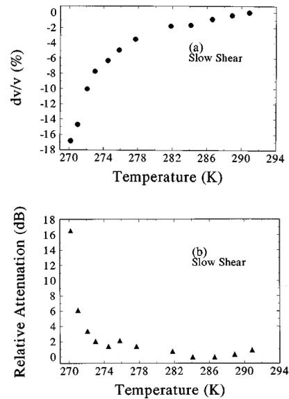
FIG. 3. Temperature dependence of the relative velocity,  $V'$  (a) and the relative attenuation (b) associated with the elastic constant  $C'$ .
