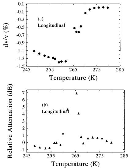
FIG. 1. Temperature dependence of the relative velocity,  $V_L$  (a) and the relative attenuation (b) associated with the elastic constant  $C_L$ .
