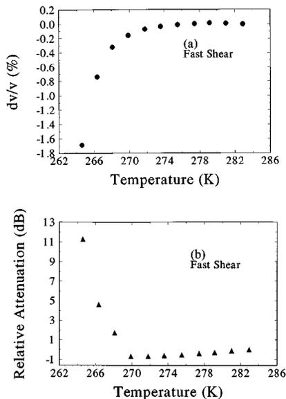
FIG. 2. Temperature dependence of the relative velocity,  $V_{44}$  (a) and the relative attenuation (b) associated with the elastic constant  $C_{44}$ .
