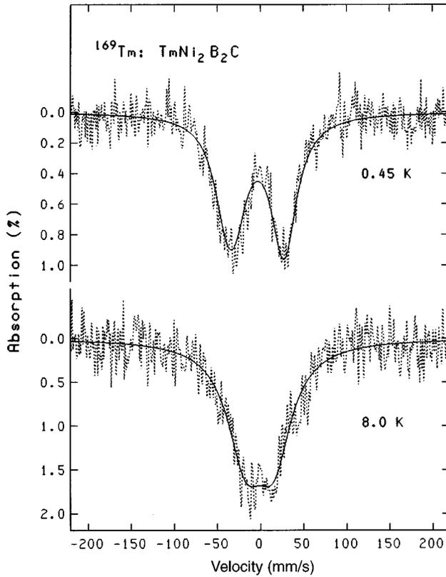
FIG. 1. Two spectra recorded below (0.45 K) and above (8 K) the transition temperature of 1 K. The 0.45 K spectrum shows a slightly broadened left Mössbauer peak indicative of a small Tm moment in the order of  $0.1\mu_B$ . Note that the QS at 0.45 K is clearly larger than at 8 K. Above 1 K a broadening of the quadrupole doublet lines is observed.
