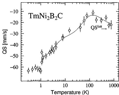
FIG. 2. The quadrupole splitting  $QS=(1/2)eV_{zz}Q$  as observed by  $^{169}\text{Tm}$  Mössbauer spectroscopy as a function of temperature. The sudden change at 1 K is related to magnetic or to quadrupolar ordering (see text). The solid curve is obtained from the crystal field parameters  $B_2^0=-1.16$  K,  $B_4^0=4.61\times 10^{-3}$  K,  $B_4^4=-0.173$  K,  $B_6^0=-1.44\times 10^{-5}$  K, and  $B_6^4=-1.11\times 10^{-3}$  K but can be considered only as a guide to the eye (see text).
