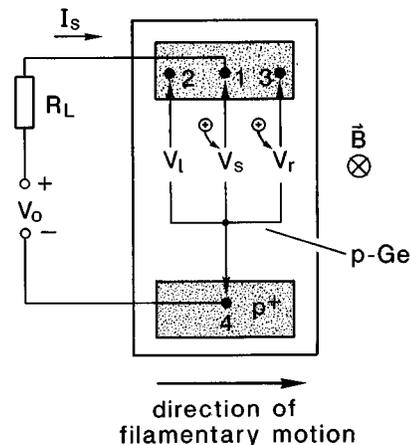
FIG. 1. The experimental setup used is similar to the one discussed elsewhere (Ref. 5), but instead of applying a constant voltage between the two planar contacts, the voltage is periodically switched on and off, in order to control the time of absence of a filament.
