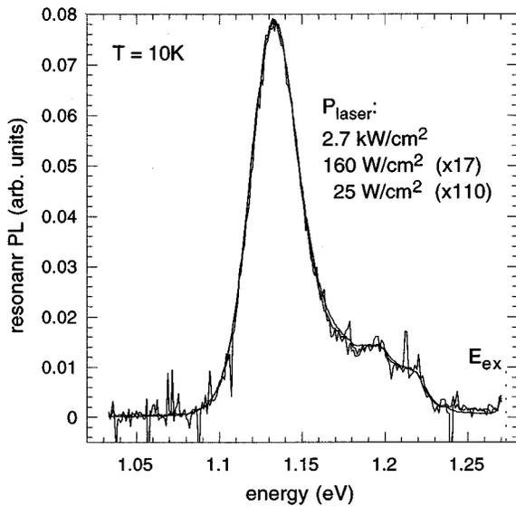
FIG. 6. RPL spectra of sample II measured at different pump intensities and with the same excitation energy  $E_{ex}$  of the Ti-sapphire laser. The spectra are normalized to the spectrum measured with the highest pump intensity (multiplication factors in brackets).
