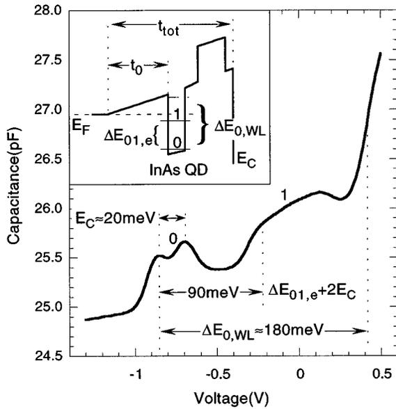
FIG. 1. Capacitance spectrum of sample I measured at  $T=4.2$  K with an ac bias of 5 mV. The inset shows a schematic conduction band diagram ( $E_C$ ) of the sample at  $U=0$  V.
