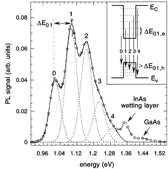
FIG. 2. PL spectrum ( $-O-O-$ ) of sample I pumped with 30 W/mm<sup>2</sup> of an Ar<sup>+</sup>-laser at  $T=300$  K. The solid line shows a Gaussian fit ( $---$ ) to the experimental data. The numbered transitions in the inset are attached to the numbered PL peaks.  $E_C$  and  $E_V$  are the conduction- and valence-band edges, respectively.
