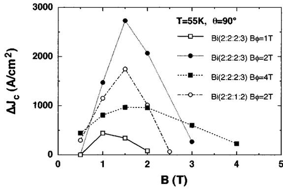
FIG. 5. The excess critical current densities  $\Delta J_c(\theta=90^\circ)$  at 55 K are plotted as a function of applied magnetic fields for the irradiated Bi(2:2:2:3) tapes for fluence  $\phi=0.5, 1.0,$  and  $2.0 \times 10^{11}$  ions/cm<sup>2</sup> and the Bi(2:2:1:2) tape for  $\phi=1.0 \times 10^{11}$  ions/cm<sup>2</sup>.
