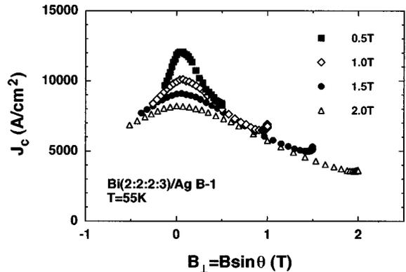
FIG. 4. The scaled critical current densities  $J_c(B_\perp)$  with the perpendicular component of the applied magnetic fields  $B_\perp$  are shown for the Bi(2:2:2:3) tape with  $B_\phi=1$  T.
