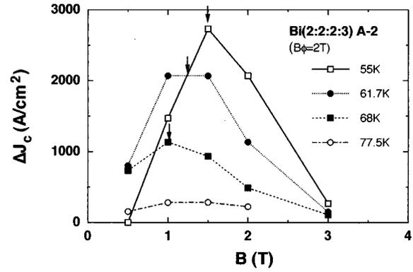
FIG. 6. The excess critical current densities  $\Delta J_c(\theta=90^\circ)$  at 55, 61.7, 68.0, and 77 K are plotted as a function of applied magnetic fields for the irradiated Bi(2:2:2:3) tapes for  $\phi=1.0 \times 10^{11}$  ions/cm<sup>2</sup>.
