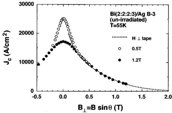
FIG. 2. The scaled critical current densities  $J_c(B_\perp)$  with the perpendicular component of the applied magnetic fields,  $B_\perp = B \sin\theta$ , are shown for the unirradiated Bi(2:2:2:3) tape.
