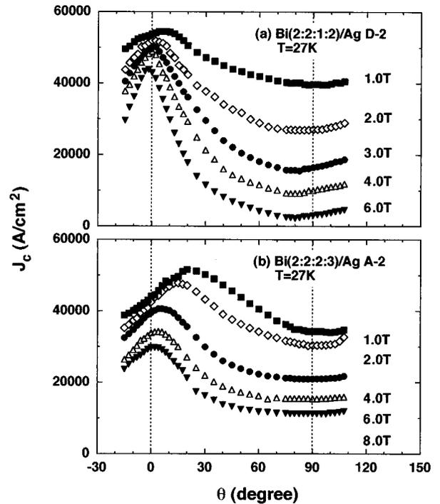
FIG. 7. The angular dependences of the critical current densities at 27 K are shown for the tapes of (a) Bi(2:2:1:2) and (b) Bi(2:2:2:3), respectively, which were irradiated to  $\phi=1.0 \times 10^{11}$  ions/cm<sup>2</sup>.
