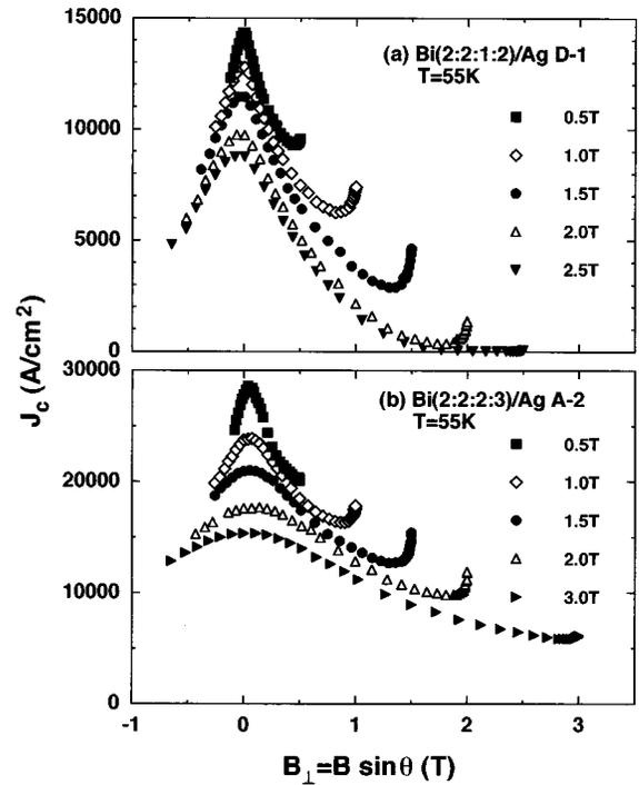
FIG. 3. The scaled critical current densities  $J_c(B_\perp)$  with the perpendicular component of the applied magnetic fields  $B_\perp$  are shown for the data in Fig. 1 for (a) Bi(2:2:1:2) and (b) Bi(2:2:2:3). Both of these were irradiated to  $B_\phi=2$  T.
