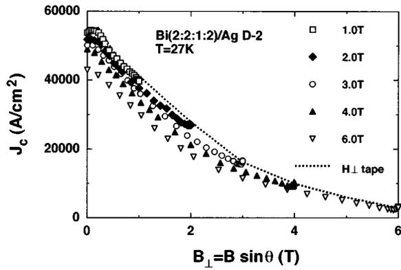
FIG. 8. The scaled critical current densities  $J_c(B_{\perp})$  for the data shown in Fig. 7 [a Bi(2:2:1:2) tape at 27 K].
