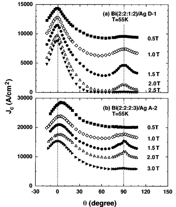
FIG. 1. The angular dependences of the critical current densities at 55 K are shown for the Ag-sheathed tapes of (a) Bi(2:2:1:2) and (b) Bi(2:2:2:3), respectively, which were irradiated with 5.8-GeV Pb ions to a fluence of  $1.0 \times 10^{11}$  ions/cm<sup>2</sup>.  $\theta$  is the angle between the direction of applied magnetic fields and the plane of the tape.
