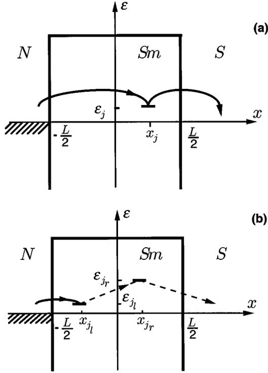
FIG. 1. Schematic picture of the  $N$ - $Sm$ - $S$  junction with (a) single localized state and (b) two-impurity chains.
