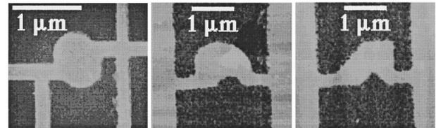
FIG. 2. Cavity images. The stadium image was obtained with a scanning electron microscope; the light areas are metal and the dark areas are the GaAs surface. The stomach and polygon images were obtained with a scanning force microscope; the light areas are unetched GaAs and the dark areas are etched to a depth of 23 nm.
