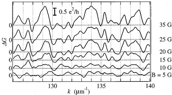
FIG. 4.  $\Delta G(k, B) \equiv G(k, B) - G(k, 0)$  for the stomach at several values of  $B$  between 0 and  $\approx \phi_0\alpha$ . The behavior of  $G(B)$  for the 25 ensemble members shown in the figure ranges from a maximum at  $B=0$  (e.g.,  $k \approx 128\text{ }\mu\text{m}^{-1}$ ) to a minimum at  $B=0$  (e.g.,  $k \approx 134\text{ }\mu\text{m}^{-1}$ ).
