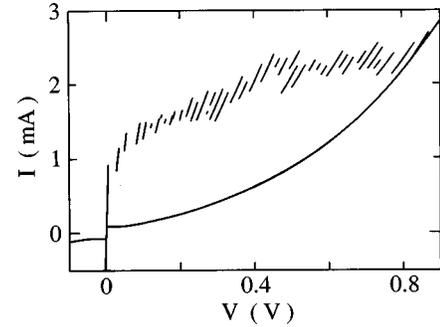
FIG. 2.  $I$ - $V$  characteristics of a 60 nm thick junction stack at 4.2 K. The  $j_c$  is 250–500 A/cm<sup>2</sup>. The  $V_c$  value is approximately 0.8 V.
