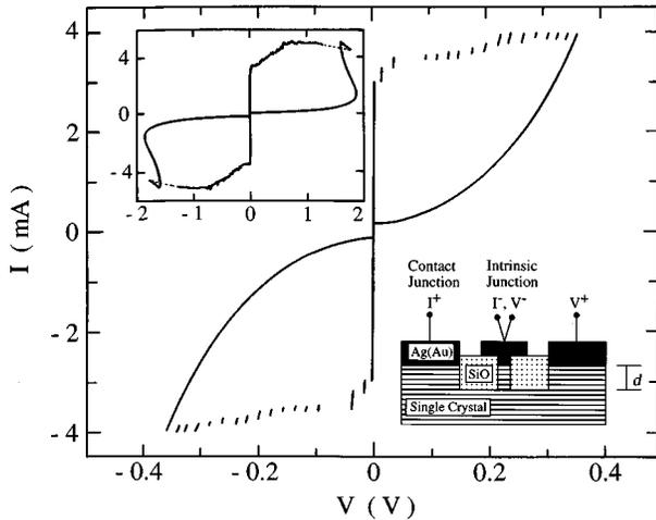
FIG. 1.  $I$ - $V$  characteristics of a 300 nm thick junction stack at 11 K. The curve for a larger bias current is indicated in the inset. The critical current density  $j_c$  is 750–1250 A/cm<sup>2</sup>. The schematic cross-sectional view of the junction stacks is also shown.
