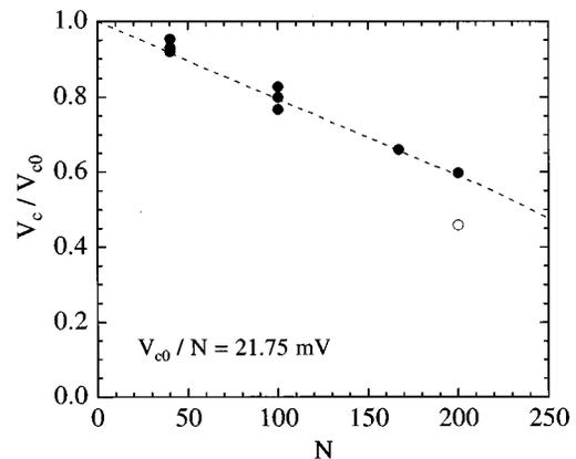
FIG. 3. Variation in characteristic voltage  $V_c$  with number of CuO<sub>2</sub> bilayers,  $N$ , contained in different junction stacks with a  $j_c$  of approximately 500 A/cm<sup>2</sup> (filled circles) and 1000 A/cm<sup>2</sup> (open circle). The  $V_c$  value is normalized by  $V_{c0} = 21.75 \times N$  mV. The broken line is the variation roughly estimated assuming nonequilibrium gap suppression based on the  $T^*$  model and a current density  $J$  of 1000 A/cm<sup>2</sup> (see text).
