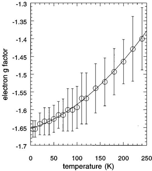
FIG. 3. Temperature dependence of the measured  $g^*$  (circles with error bars) and an empirical fit by the equation  $g^*(T) = -1.653 + 4 \times 10^{-4} T + 2.8 \times 10^{-6} T^2$  (solid curve).
