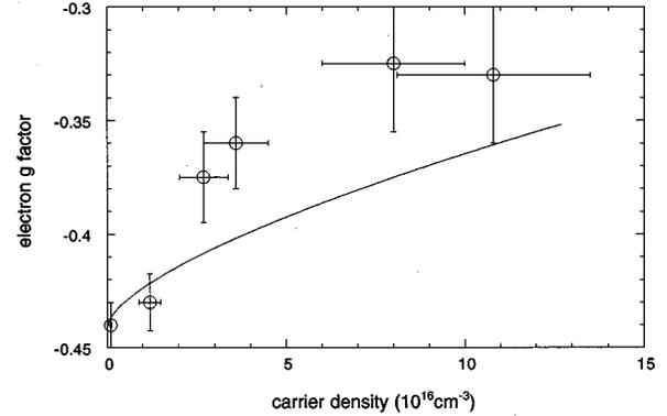
FIG. 7. Dependence of  $g^*$  on the excitation density. The open circles are measured and the solid line is the calculated  $g^*$  at the Fermi edge. The experimental densities are determined by a line-shape analysis of the transient spectra.
