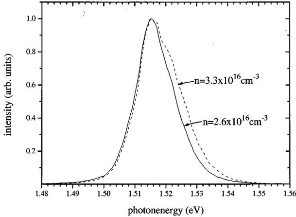
FIG. 6. Right and left circularly detected PL spectra. The spectra are measured one spin quantum beat oscillation period after excitation at a lattice temperature of 20 K and demonstrate two different Fermi-Dirac distributions for spin-up and spin-down electrons. A line-shape analysis yields the two different carrier densities.
