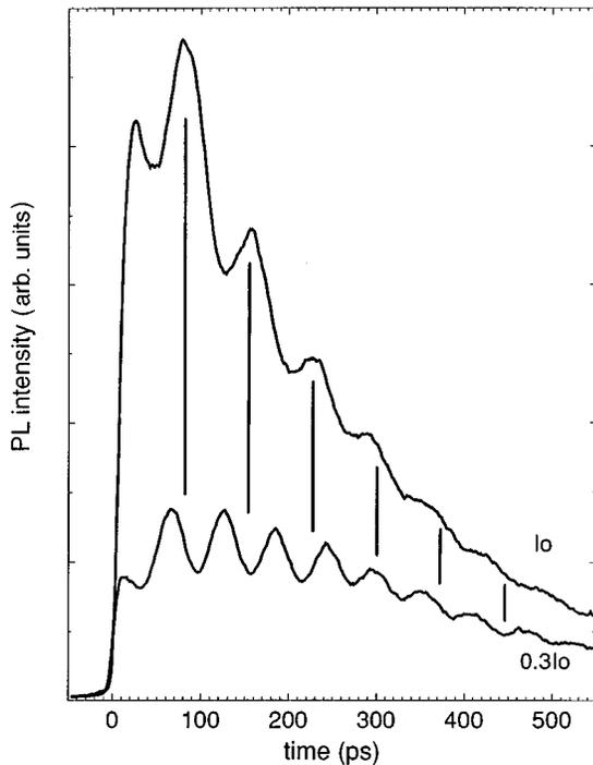
FIG. 4. Circularly polarized detected PL in bulk GaAs at two different excitation densities ( $I_0, 0.3I_0$ ) after circularly polarized excitation in the continuum at a magnetic field of 3 T. The different oscillation periods of the PL directly demonstrate the density dependence of the average  $g^*$ . The vertical solid lines are guides to the eye to illustrate the phase shifting. The excitation density at  $I_0$  is  $8 \times 10^{16} \text{ cm}^{-3}$ .
