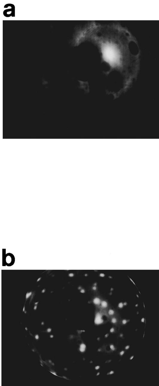
FIG. 1. (a) Diffuse ring observed in the LEED pattern of 1 ML of C<sub>60</sub> on Pt(111) at  $T < 770$  K. The spot at the center of the ring is the (00) beam and the primary energy  $E_p$  is 20 eV. (b) LEED pattern of the well-ordered C<sub>60</sub> monolayer obtained after annealing at  $T > 900$  K at  $E_p = 26$  eV.
