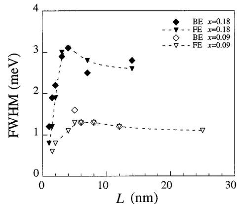
FIG. 5. FWHM of the HHFE and  $BE_i$  luminescence vs the well width for  $x = 0.09$  and  $x = 0.18$ .
