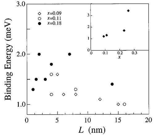
FIG. 4. Binding energy of the  $BE_i$  state measured with respect to the HHFE state for samples with  $x = 0.09, 0.11,$  and  $0.18$ . In the inset, the  $BE_i$  binding energy at fixed well width  $L = 8$  nm is reported vs indium concentration  $x$ .
