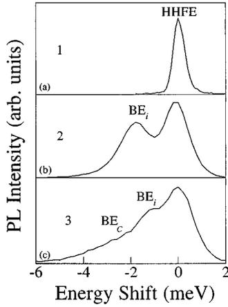
FIG. 1. Photoluminescence at  $T = 5$  K of three different quantum wells. The energy is measured with respect to that of the HHFE: (a)  $x = 0.09$ ,  $L = 1.5$  nm, undoped (HHFE peak energy = 1.504 eV); (b)  $x = 0.11$ ,  $L = 4.0$  nm, undoped (HHFE peak energy = 1.468 eV); (c)  $x = 0.10$ ,  $L = 20$  nm, C doped (HHFE peak energy = 1.444 eV).
