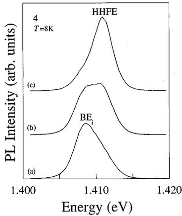
FIG. 3. Photoluminescence spectra of a quantum well with  $x = 0.185$  and  $L = 4$  nm (sample 4) for three different values of the excitation energy  $E_{\text{exc}}$ . (a)  $E_{\text{exc}} = 1.473$  eV; (b)  $E_{\text{exc}} = 1.467$  eV; (c)  $E_{\text{exc}} = 1.463$  eV.
