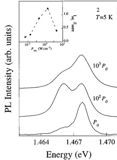
FIG. 2. Photoluminescence spectra of a quantum well with  $x = 0.11$ ,  $L = 4$  nm for different values of the exciting power density  $P_{\text{exc}}$ .  $P_0 = 2 \times 10^{-2}$  W cm $^{-2}$ . The ratio between the integrated intensities of the  $\text{BE}_i$  and HHFE recombinations is reported in the inset vs  $P_{\text{exc}}$ .
