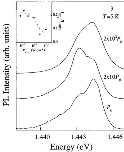
FIG. 6. Photoluminescence spectra of a quantum well with  $x = 0.10$ ,  $L = 10$  nm for different values of the exciting power density.  $P_0 = 5 \times 10^{-4}$  W cm $^{-2}$ . The ratio between the integrated intensities of the BE $_C$  and HHFE recombinations is reported in the inset vs  $P_{\text{exc}}$ .
