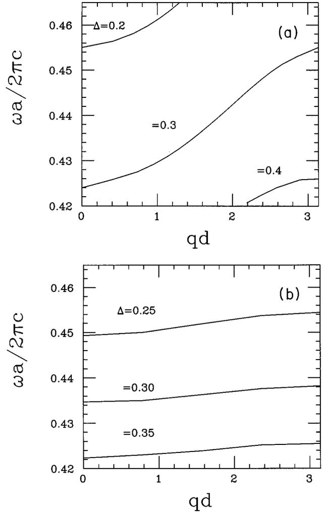
FIG. 2. Plot of  $\omega/c$  versus  $qd$  for (a)  $\mathbf{S}_{1,0}$  and (b)  $\mathbf{S}_{1,1}$ . Curves are labeled as states of constant  $\Delta$ . All lengths are measured in units of  $a$ .
