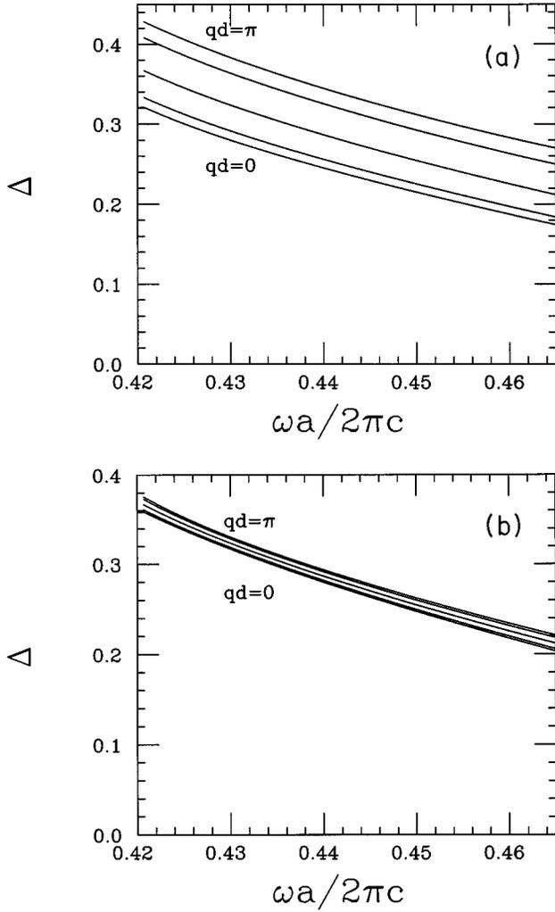
FIG. 1. Plot of  $\Delta$  versus  $\omega/c$  for (a)  $\mathbf{S}_{1,0}$  and (b)  $\mathbf{S}_{1,1}$ . Curves are labeled from bottom to top as  $qd=0, \pi/4, \pi/2, 3\pi/4, \pi$ . All lengths are measured in units of  $a$ .
