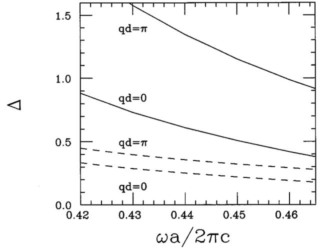
FIG. 4. Plot of  $\Delta$  versus  $\omega/c$  for  $t=0.01a$  (dashed) and  $t=0.1a$  (solid). Curves of  $qd=0$  and  $qd=\pi$  are labeled. For each  $t$ , the curves for  $0 < qd < \pi$  fall between the  $qd=0$  and  $qd=\pi$  limits. All lengths are measured in units of  $a$ .
