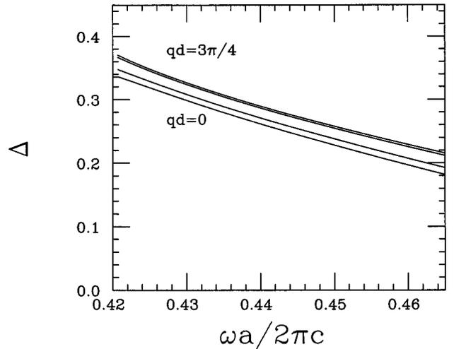
FIG. 5. Plot of  $\Delta$  versus  $\omega/c$  for the two-dimensional impurity array described in the text. The curves are labeled bottom to top as states of  $qd=0, \pi/4, \pi/2, \pi$ , and  $3\pi/4$ . (Note: The curves for  $qd=\pi/2$  and  $\pi$  coincide.) All lengths are measured in units of  $a$ .
