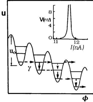
FIG. 1. Potential  $U(\phi)$  describing the junction dynamics. A sharp voltage peak in the  $I$ - $V$  characteristics appears when the ground state lies on an energy level very close to one of the first excited states in the next well; this is shown in the inset for the following junction parameters:  $E_0/\hbar\omega_j=2.5$ ,  $T=50$  mK,  $I_c=200$  nA, and  $R/R_Q=100$ , where  $R_Q=\pi\hbar/2e^2=6.45$  k $\Omega$ .
