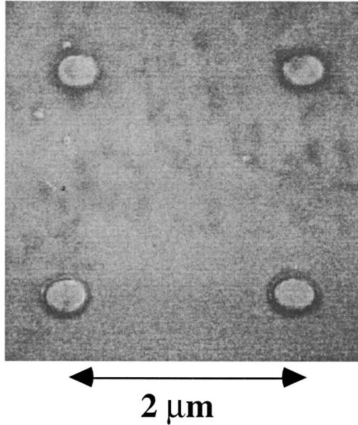
FIG. 1. Electron micrograph showing four Co particles (ellipticity  $300\text{ nm}\times 200\text{ nm}$ , thickness  $35\text{ nm}$ ) belonging to an array of step  $2000\text{ nm}$ .
