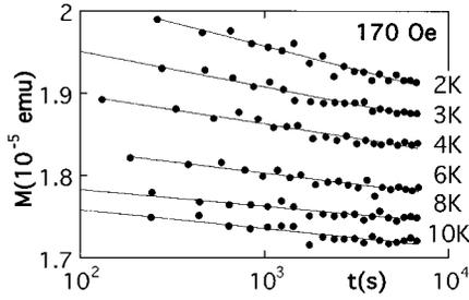
FIG. 3. Relaxation of magnetization of the array of Co particles at  $H = 170$  Oe. The slope  $S = dM/d(\ln(t))$  defines the magnetic viscosity.
