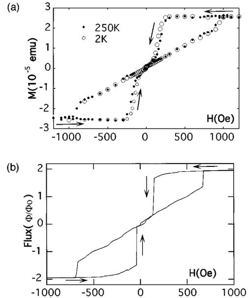
FIG. 2. (a) Hysteresis cycles of the array of about  $2\times 10^7$  Co particles ( $300\text{ nm}\times 200\text{ nm}\times 30\text{ nm}$ ) measured at  $2\text{ K}$  ( $\circ$ ) and  $250\text{ K}$  ( $\bullet$ ). The in-plane field is applied along the long axis of the particles. (b) Hysteresis loop of a single Co particle of same dimension.
